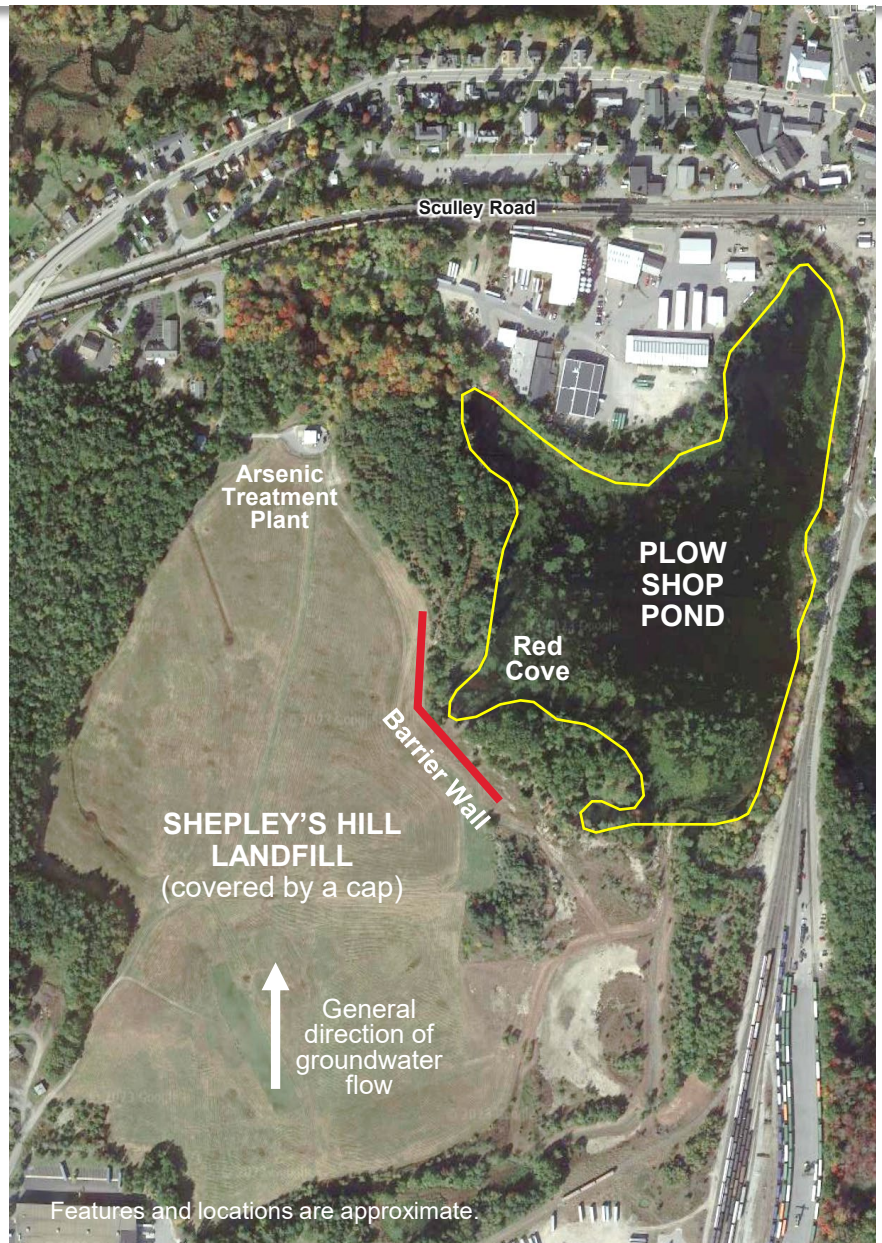
Right: Map of the area to show the location of Shepley's Hill Landfill, Plow Shop Pond, the groundwater barrier wall, and the Army's existing arsenic treatment plant. Extraction wells capture groundwater that is then pumped to the plant to remove arsenic.
